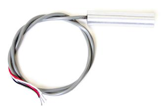
The Model 12 Air Temperature Sensor (P/N 10-70-7483) is intended for use in applications that monitor slowly changing temperatures. The unit gives approximately .5 °F (.25 °C) resolution when used with an 8-bit analog input.
